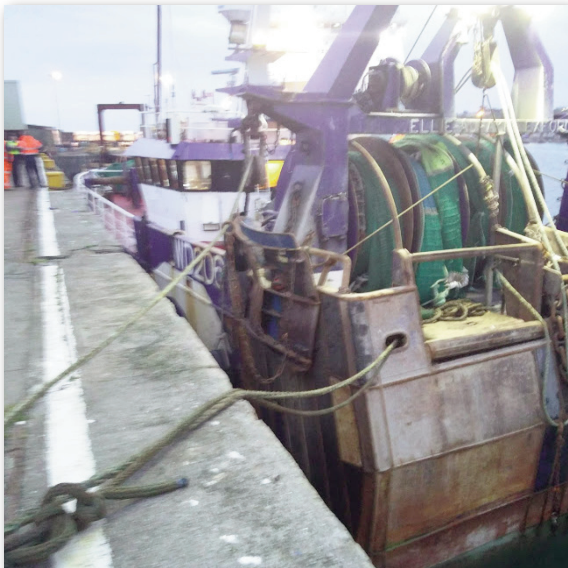
Photograph No. 1. Mooring lines from the 'MFV Ellie Adhamh' to the quay wall.
